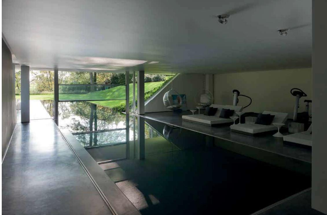
The building yields to the wishes of its occupiers. A movable wall can separate the indoor pool from the outdoor pool. The floor can also be raised to cover the water, creating a large area for hosting friends.
